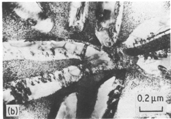
Figure 7 Ti-10V, \beta -solutionized and isothermally reacted at (a) 873 K for 1 h showing the typical \alpha/\beta interface and (b) 948 K for 1 h showing predominantly type 1 \alpha -plates distributed in a \beta - \omega matrix.
